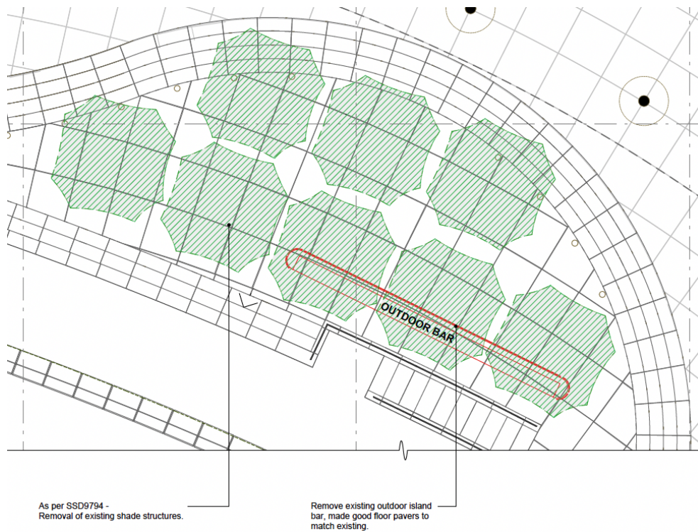
Figure 8: Extract from LK drawing DA-100 showing location and demolition of existing timber clad outdoor island bar (shown in red) as proposed in this SSD-9794 Mod 1 application. The existing umbrellas, shaded green, were previously approved for removal and replacement as part of SSD-9794.
